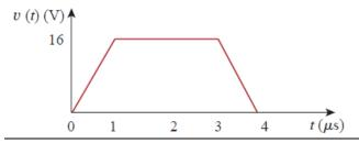
**6.11** A 4-mF capacitor has the current waveform shown in Fig. 6.48. Assuming that sketch the voltage waveform v(t).
